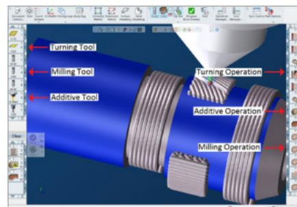
Turning, milling, and additive tools and operations in GibbsCAM 14
